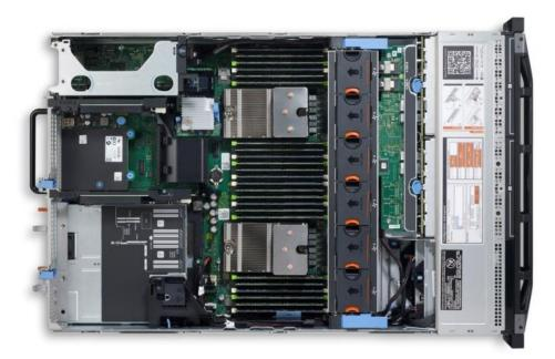
Figure 7. R720 internal chassis view
